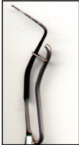
Figure 2 - A sample of the pressure controlled probe with a stop at 0.25N.
