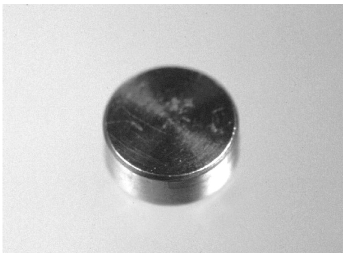
FIGURE 1 – Picture of the implant prototype. Disc of Ti cp – 4.76 mm of diameter and 2 mm wide.
