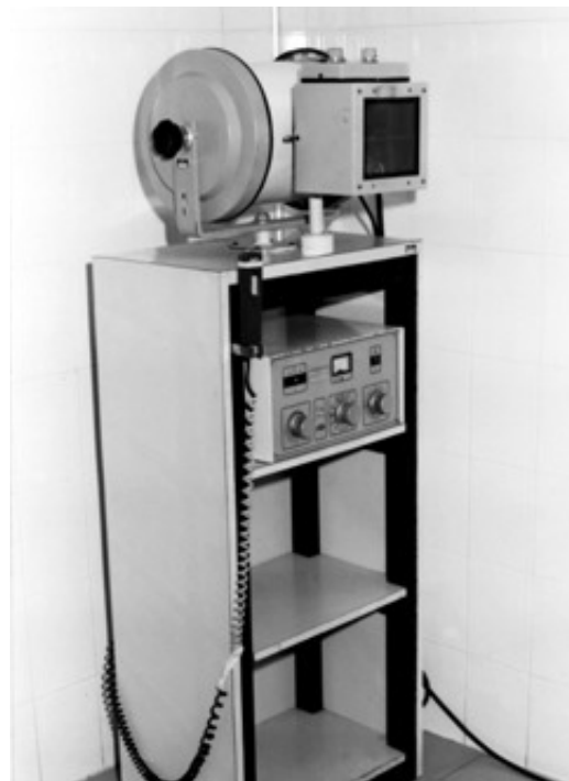
FIGURE 1 – The adapted radiologic system with a 100 mA, 90 KVp Roentax 100 tube (Emic, São Paulo) assembled in a wood base covered with formica connected to a light system of bundle direction.
