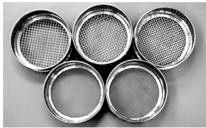
FIGURE 4 - System of silk sieves with orifices measuring 1.2, 2.83, 4 and 4.75 mm.
